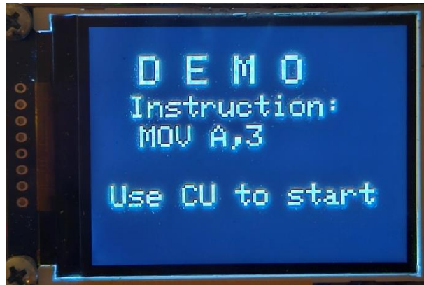
Fig. 5.6 The instruction MOV A,3 will be loaded in memory
