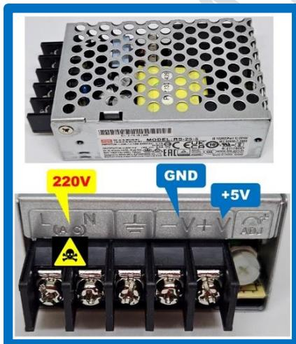
**Fig. 4.3** External power supply (PS)
