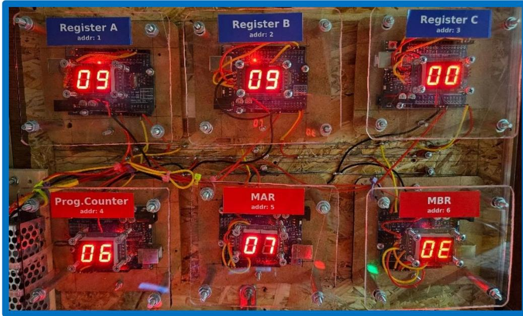
Fig. 3.6 Preparation (MAR) for fetching the second byte of the instruction
